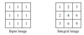
Fig5. Transform Input image to Integral image
